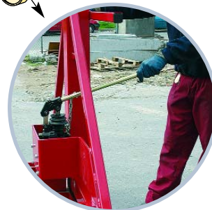
CLOSE-UP THE HYDRAULIC SYSTEM FOR LIFTING AND LOWERING
